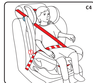
Step 3: Put the child in the seat and follow C3, C4, C5 routine to install.
