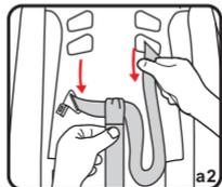
Make sure that both of the shoulder belts and chest belt go through slots at the same height, and not twisted.
