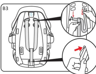
**Step 3:** Pull out the buckle tongues from the chestpad and the slots on the cover (B3)
