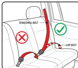
Only suitable if the approved vehicles are fitted with 3 point safety-belts, approved to UN/ECE Regulation No.16 or other equivalent standards.
