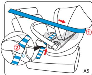
**Step 5:** Pull out the 3-point car seat belt, through the belt route slot of backrest follow the routine ①②③(A5、A6、A7)
