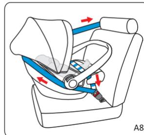
**Step 7:** Pull car seat belt follow the direction of red arrow and make sure the belt is tight enough(A8).
