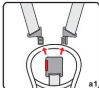
**Step 2.** Pull out the buckle tongues from the chest pad and the slots on the cover(a2). and the shell then thread them into the corresponding belt slots(a3).
