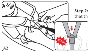
**Step 2:** Fasten the harness. Check that the harness does not twisted.
