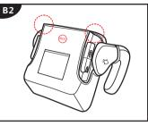
Step1: Press the button on the bottom and turn isofit connector to hide.
