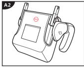
Step 1: Turn the seat to the bottom and pull out isofix connector. (A1, A2)
