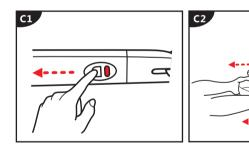
**Step 1:** Pull child seat forward and slide the locking system. When you hear "click" and it turns to red, isofix connector is released. Step 2: Take child seat away from car seat.
