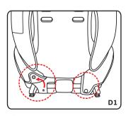
**Step 1:**Turn the seat to the back and unlock the snap fastener.
