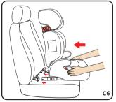
**Step 5:** Push child seat follow the direction and insert isofit connector into isofix guide.
