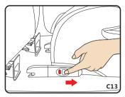
**Step 11:** Pull child seat forward and slide the locking system. When you hear "click" and it turns to red, isofit connector is released.
