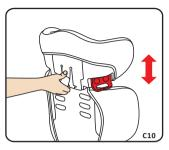
Step 9: Adjust the height of headrest and belt slot to suitable height of child(C10、C11)
