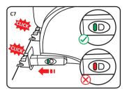
**Step 6:** Check if isofit locking system turns to green and make sure child seat is firmly connected.
