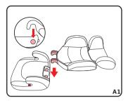
**Step 1:**Align base and backrest in a straight line.
