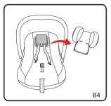
**Step 4:** Unbutton the cloth cover and remove the headrest(B4).
