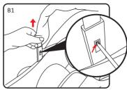
**Step 1:** The canopy can be removed by withdrawing the awning strip from the clamping groove with tools(B1).
