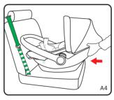
Step 4: Place the child seat on the car seat rearward-facing and make sure that the front of the child seat is firmly pressed against the car seat backrest.
