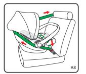
Step 7: Pull car seat belt follow the direction of red arrow and make sure the belt is tight enough(A8).
