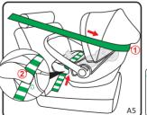
Step 5: Pull out the 3-point car seat belt, through the belt route slot of backrest follow the routine (1)(2)(3)(A5, A6, A7)
